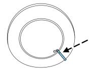
Use a tire gauge to check the tire inflation pressure, including the spare (if equipped), at least monthly and before long trips. You are strongly urged to buy a reliable tire pressure gauge, as automatic service station
